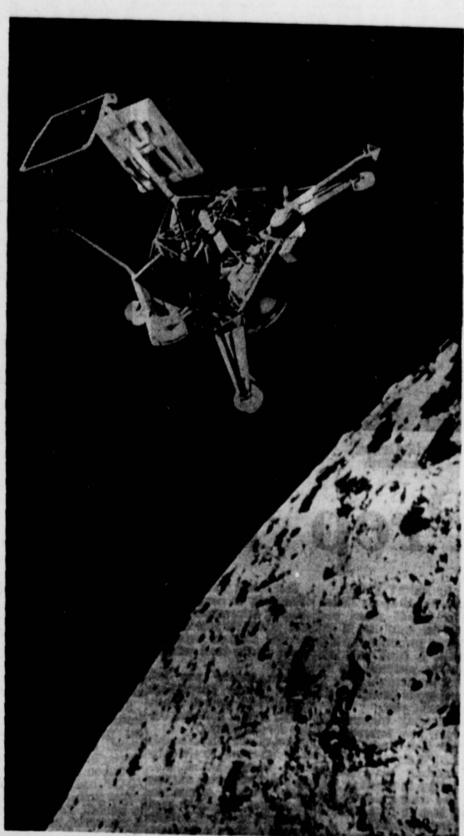
READY TO LAND . . . Hi-Shear separation nut released the Surveyor rocket, which extends between the spacecraft's legs, just before it touches down. This artist's rendition shows the Surveyor as it approached the moon at 5800 miles per hour just prior to retro-rocket ignition. This braking action slowed the rocket to achieve a soft landing on the moon.
