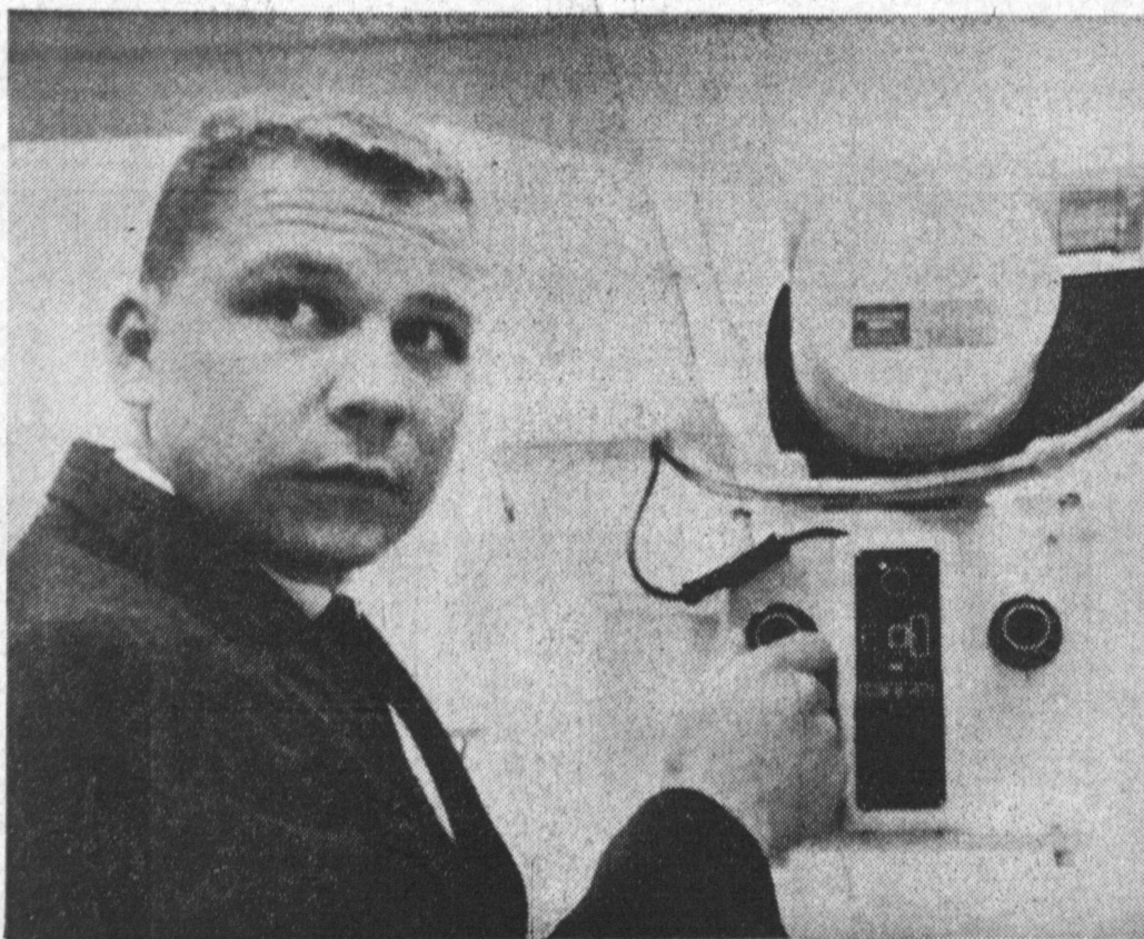
WALTER JACOBSON, supervisor of technical operations in radiology, Harbor General Hospital, explaining operation of a collimator, a device for adjusting size of x-ray beams.
