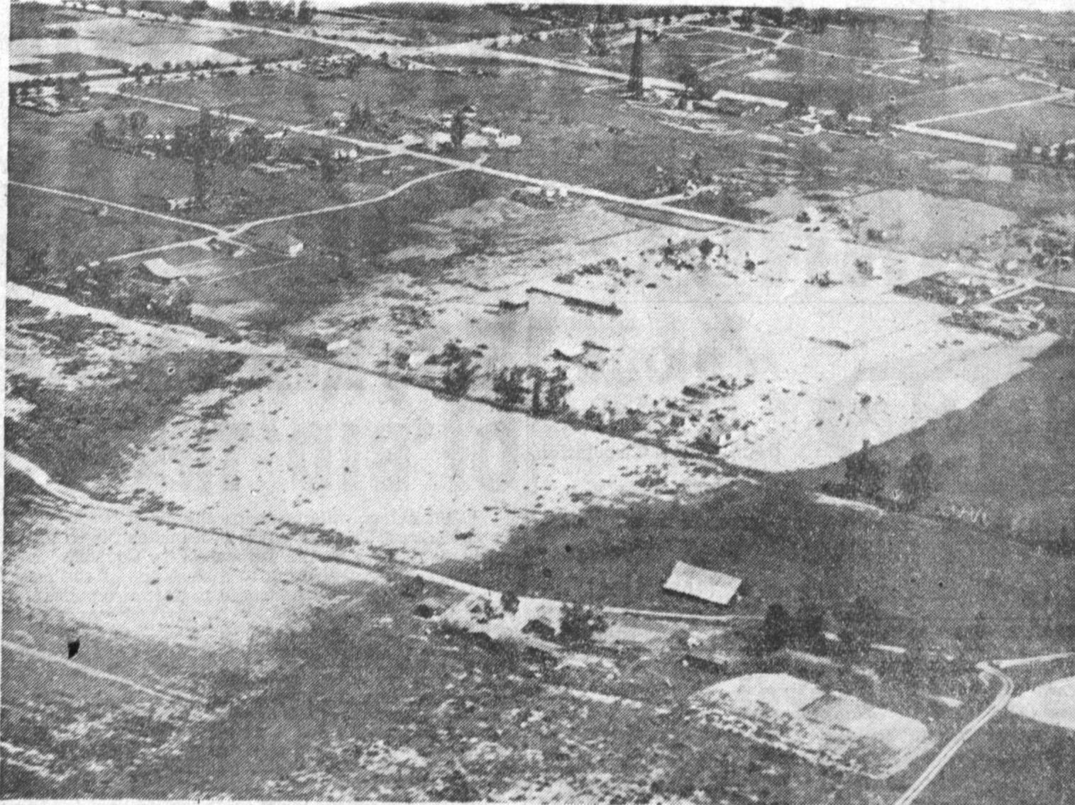
City workers have lowered the level of "Lake Walteria" by pumping out more than 1,000,000 gallons during the past several days. This view, taken from a plane piloted by Ed Dietrich of Torrance Municipal Airport, shows where a half dozen homes have been inundated, forcing most of the families to vacate. The water that is being removed is being piped to a near-by pastureland where it is absorbed into the earth. It has been suggested that owners of the tract might reduce future inundation by drilling a series of holes through the hard surface soil so that flood waters settling there might be more quickly absorbed.
