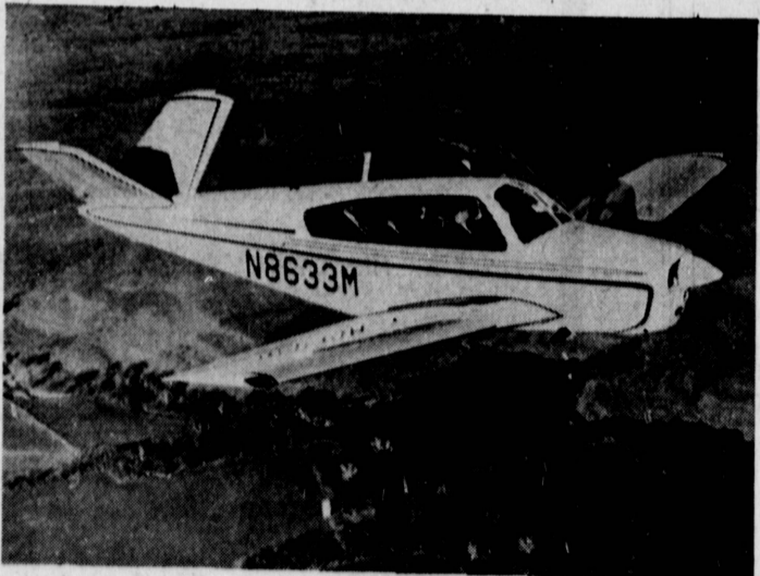
BEECHCRAFT BONANZA, all metal, four-place model 35. Top speed 212 m.p.h., range 1,145 miles. (maximum range computed without allowance for fuel used during warm-up, taxi, take-off and climb to altitude — includes 45-minute fuel reserve at maximum range speed) Tanger Aviation Sales is the local agency for the Beechcraft Bonanza.
