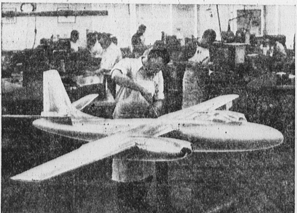
$100,000 "TOY" —This airplane model looks as if it might be a toy, but its purpose is deadly serious. It is used in high-speed wind tunnel tests, hence must be accurate to 10 thousandths of an inch. The constant improvement in North American planes creates good jobs for skilled craftsmen. To find and hold good men, North American pays good wages, encourages brains and skill with promotions to better jobs.
